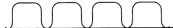
Figure 18-35. The closer the profile of the RF pulse (actually its FT) is to a rectangle, the better we can achieve contiguous slices without encountering cross-talk.
